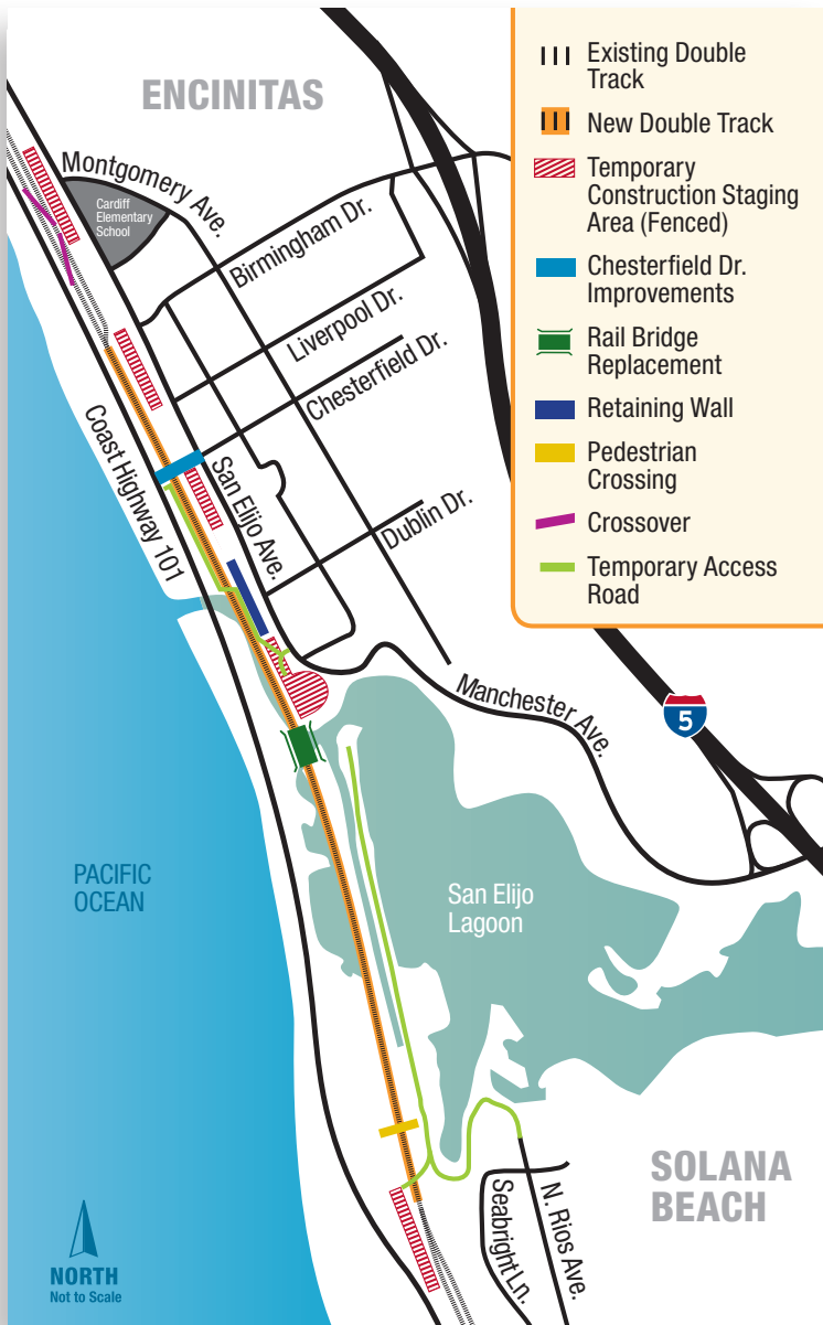
The project added 1.5 miles of second main track and replaced an aging timber rail bridge on the LOSSAN coastal rail corridor between the cities of Encinitas and Solana Beach.
