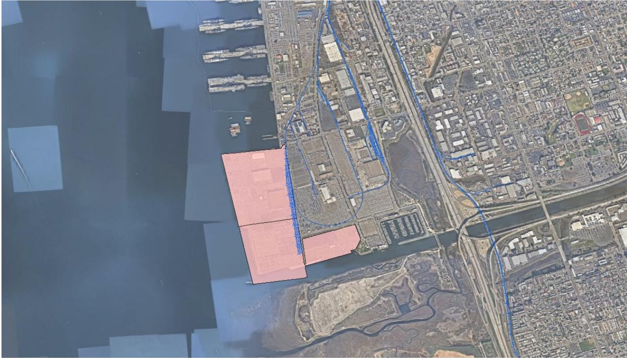
Goods move in and out of the Port by road or by rail. TAMT and NCMT both have on site rail. TAMT rail assets are owned and maintained by the Port of San Diego, rail assets at NCMT are owned by the Port of San Diego but maintained by BNSF Railway. All rail services to and from the two terminals are operated by BNSF Railway.
