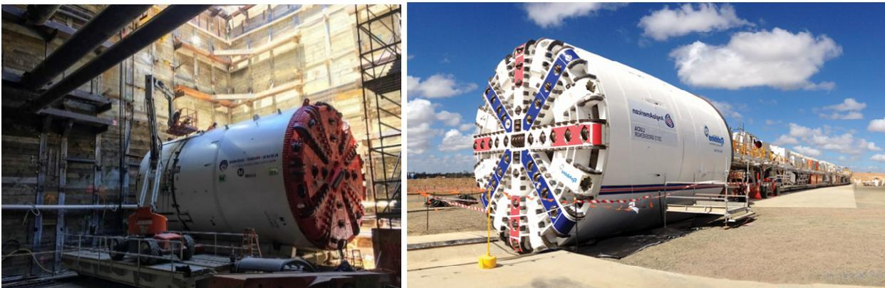
Figure 6.3. EPB TBM (left TBM, right TBM with full backup)
