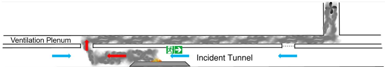
Figure 8.12. Single Point Extraction Ventilation Method
