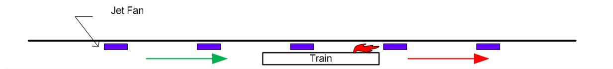
**Figure 8.6. Jet Fan Schematic, Tunnel Section View**
