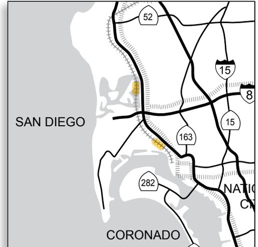
to meet and pass. The double crossover will create a virtual siding, capable of holding a full-length freight train for short periods of time.
