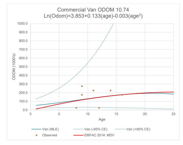
Figure 20. Commercial van odometer data
