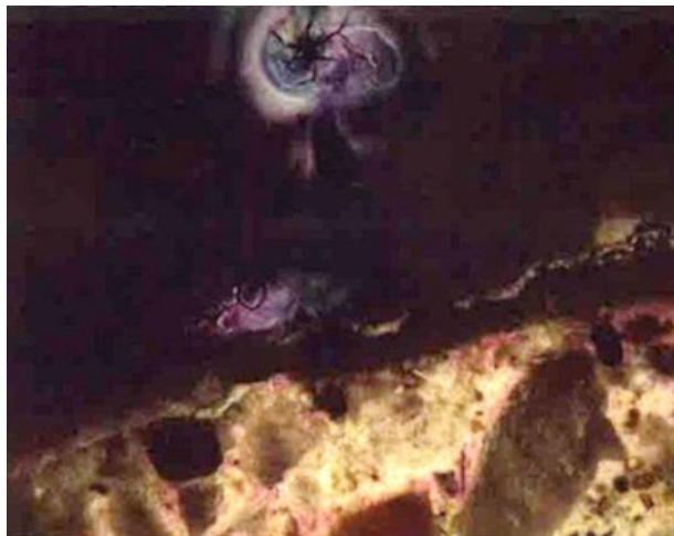
Figure 5 - Evidence of ASR in Br 225.3 pier 2
