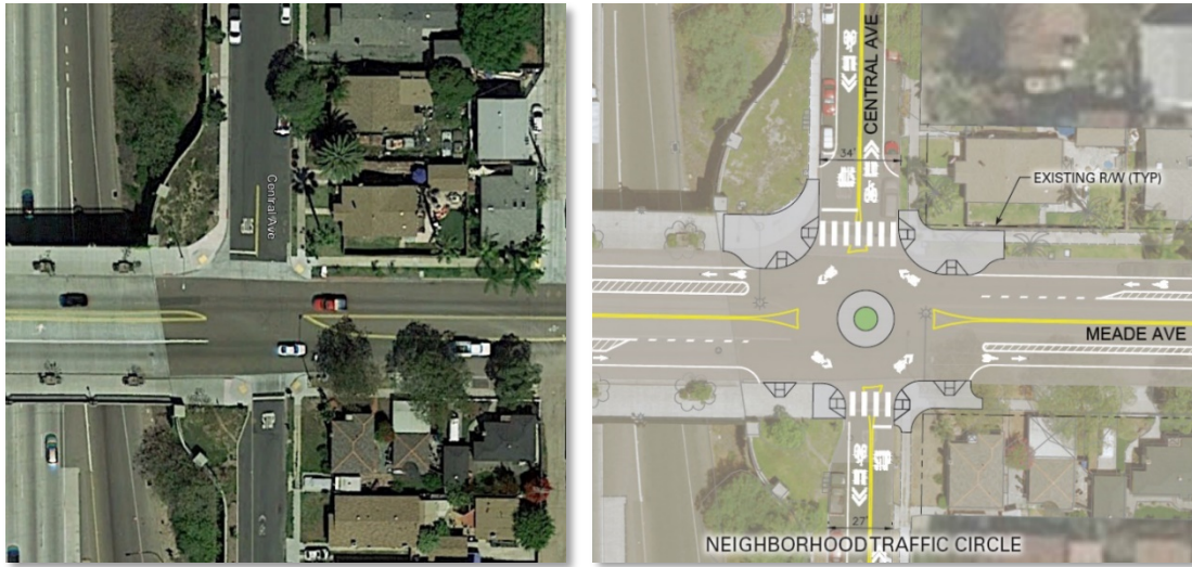
Figure 8 – Example of a bicycle and pedestrian intersection as shown by the existing intersection configuration and the proposed roundabout improvement at Central Avenue and Meade Avenue
