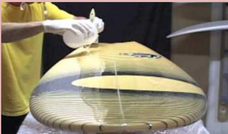
Surfboard manufacturers typically use various types of polyester resins.
