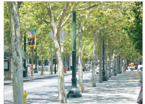
Street trees can contribute to traffic calming by defining a strong edge for the street, as shown in this example from San Jose, California.
