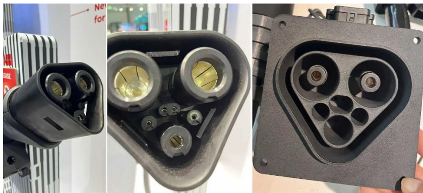
Figure 18. The Megawatt Charging System (MCS) Connector
