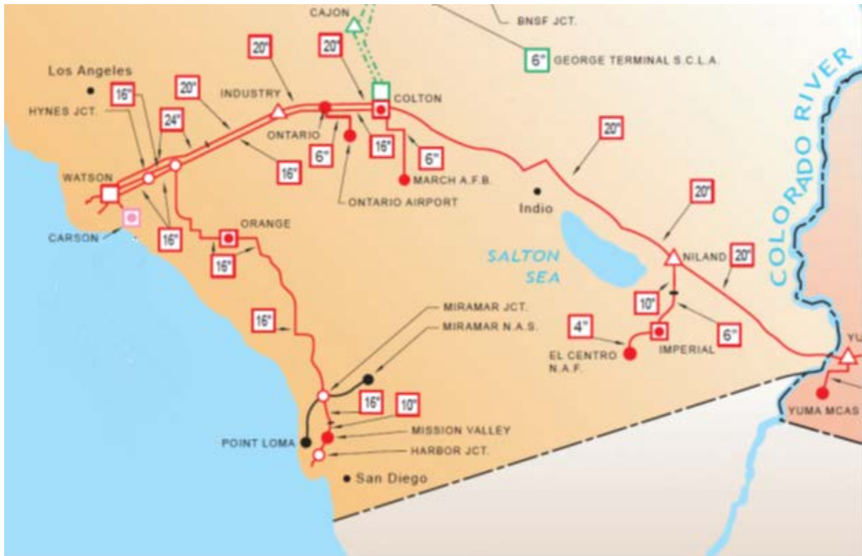
Figure 2.10: Pipeline System in Southern California
