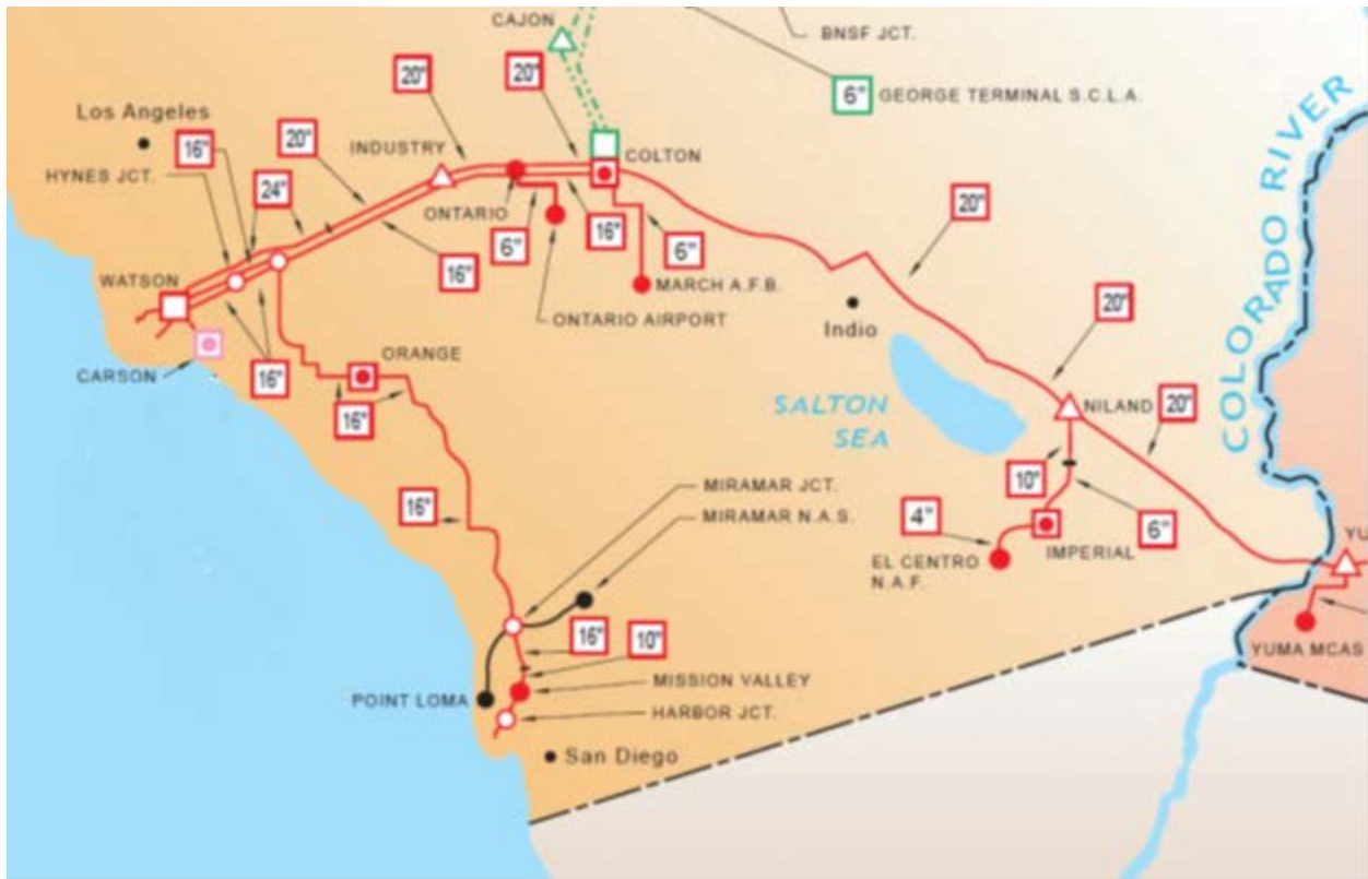
Figure 2.15: Pipeline System in Southern California
